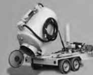
Directional Drill Mud Vacuum
